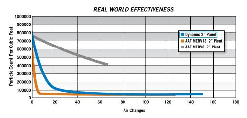
As shown above, a Dynamic 2" Panel Air Cleaner provides comparable effectiveness to a MERV 13 conventional filter, while holding almost four times the dust (below)
